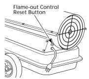
Figure 5 - Flame-out Control Reset Button
